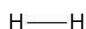
Figure 2.3A Notice that when two hydrogen atoms share a pair of electrons between them, neither takes on a charge. This is because the sharing is equal. This is called a non-polar covalent bond
